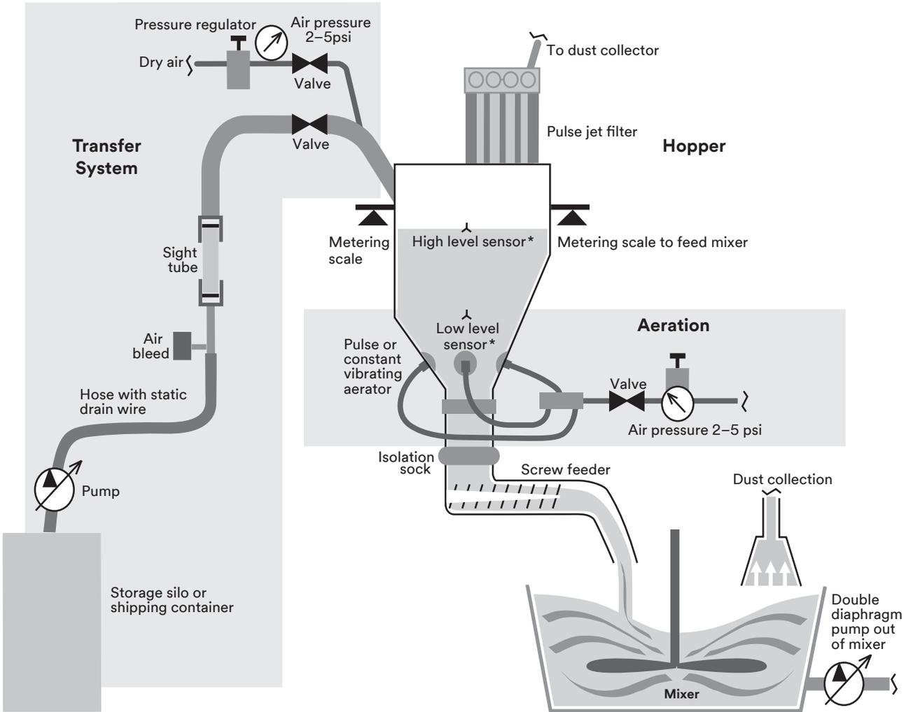
\* Signals vacuum transfer system to replenish hopper
